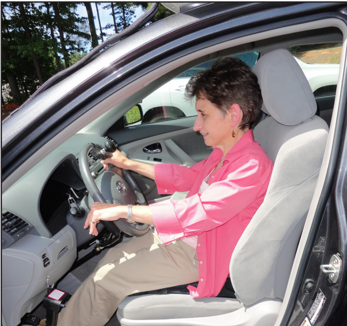
Annette Lauber demonstrates the hand controls installed in her car. This type of assistive technology can allow people with mobility disabilities to drive and travel independently.
